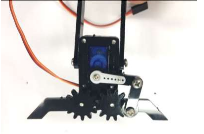
Pull the claws widely open and then insert the short arm we created in the last step and screw it firmly.
