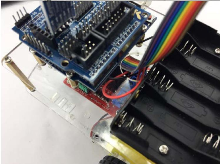
Then pull the eight jumper cables through the hole of top chassis.
