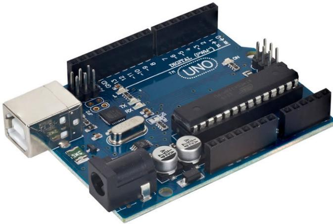
The iDuino Uno is on the ATmega328. It has 14 digital input/output pins (of which 6 can be used as PWM outputs), 6 analogue inputs, a 16 MHz ceramic resonator, a USB connection, a power jack, an ICSP header, and a reset button.
