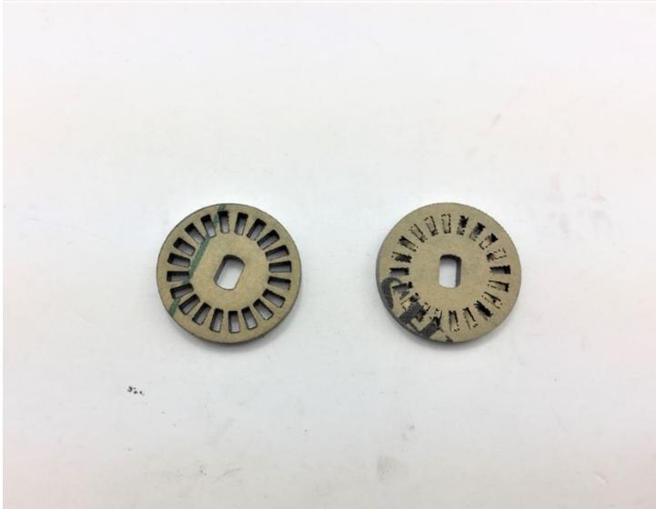
Although these two encoders included in the kit is not used, they are useful to modulate and control the speed of two motors.
