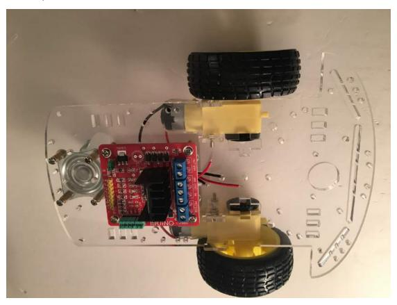
Then connect the L298N module with the motor, please note which wire should be fixed on which screw, the red wire is VCC and the black wire is GND.
