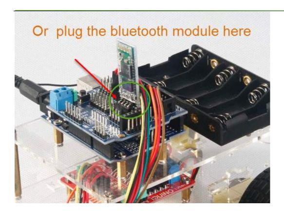
After the connection, upload the following code to your UNO board. Then power on the uno board and L298N module.
