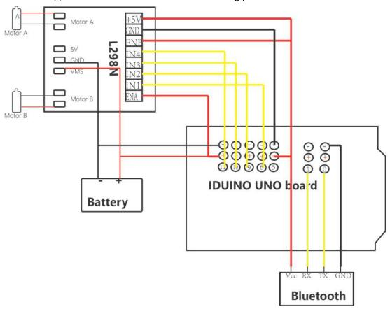
For the Bluetooth module, you can directly plug into the sensor extension board as the below picture show.
