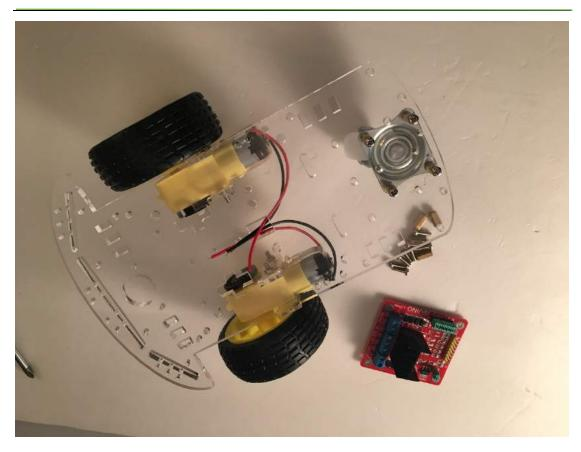
Before you fix the screw, passing the wire on the motor through the board helps your next step.
