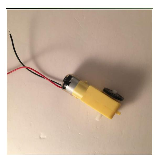
Second, use 2 fasteners to fix one motor on the bottom board. Please note which hole should be used and the motor's direction should be forward.
