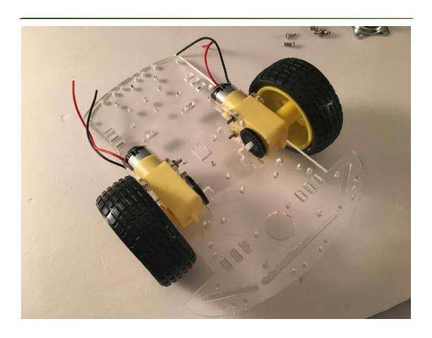
Then, install the universal wheel, please note which hole should be used on the board.
