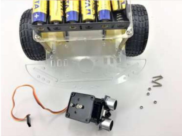
Gather four M2.5 screws and corresponding nuts in the FPV package to secure to the bottom chassis
