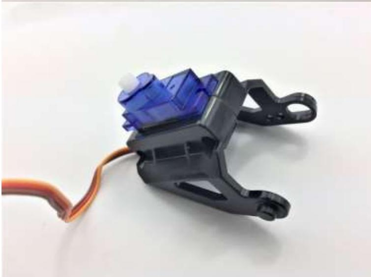
Assemble the FPV holder and servo
