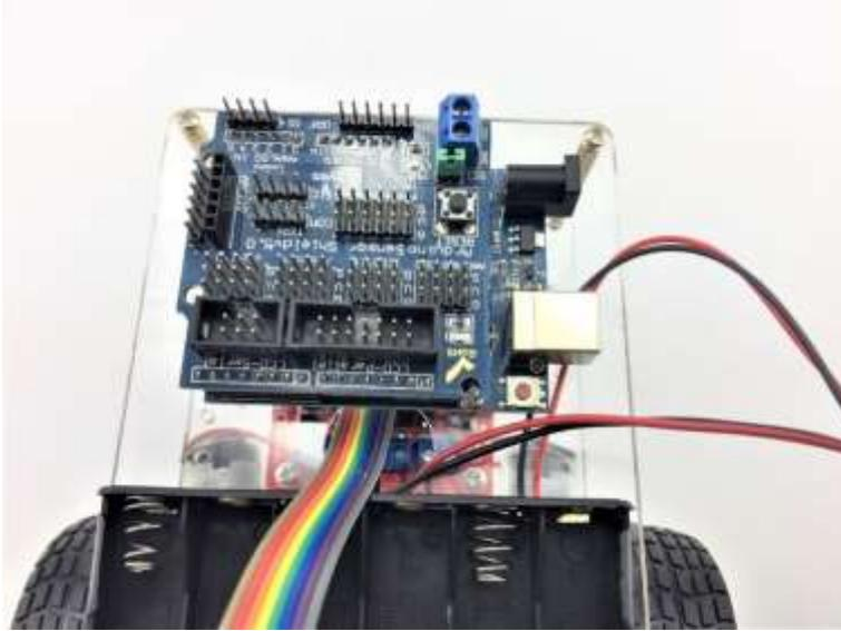
Place the sensor shield on the top of the UNO board and ensure the pins line up with the Uno Board.
