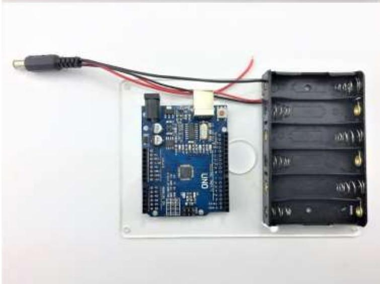
Place the battery pack and UNO board on the top acrylic chassis
