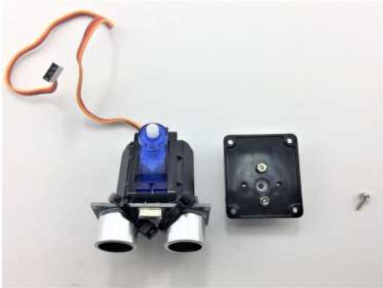
Prepare the Self-tapping screw in the Servo package and tighten the sensor part with servo rack
