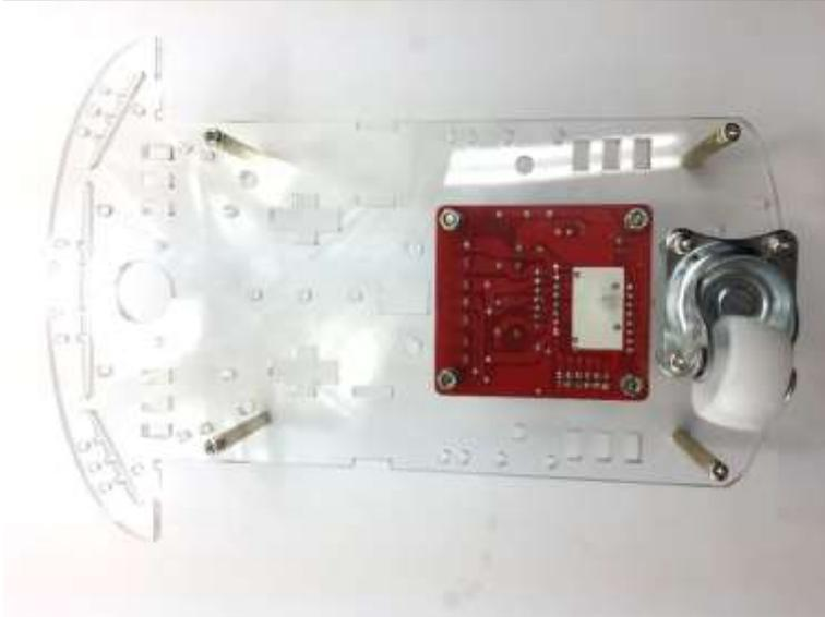
Secure Spacers onto the chassis as per the picture on the left.
