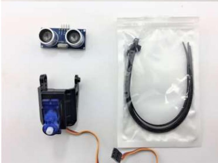
To tighten the ultrasonic sensor, we can use several cable ties (Not included in the Kit). Alternatively, you can use other methods:
