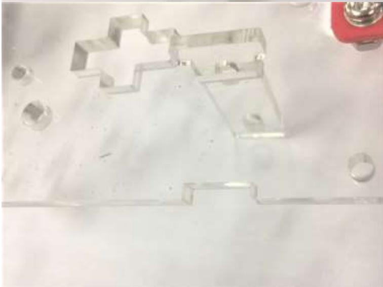
Insert the acrylic fasteners first in pre-cut slot
