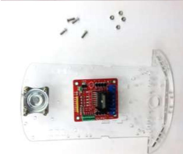
Gather 4 x M3 10mm screws and nuts to secure L289N Motor Drive board
