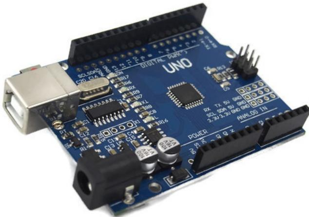
The Iduino Uno is on the ATmega328. It has 14 digital input/output pins (of which 6 can be used as PWM outputs), 6 analogue inputs, a 16 MHz ceramic resonator, a USB connection, a power jack, an ICSP header, and a reset button.
