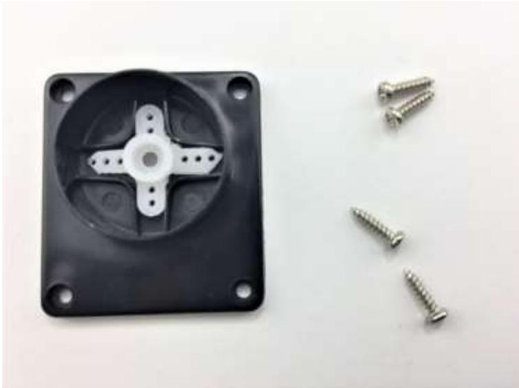
Place the modified servo horn inside the bracket and secure with 6 \* M2.5 screws in the servo package
