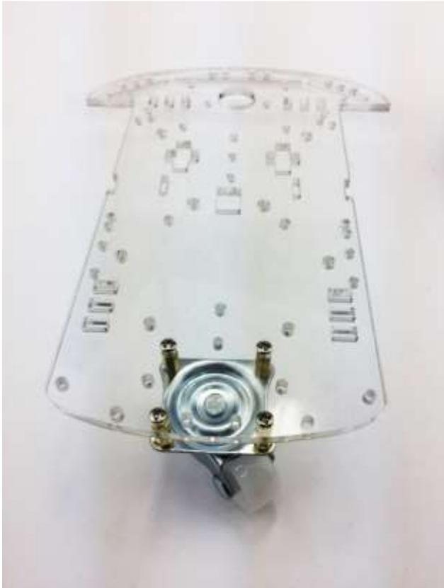
Screw in the metal pivot wheel to the chassis
