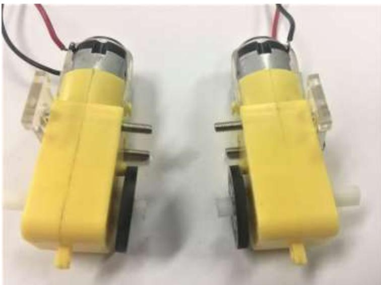
Place acrylic DC motor Brackets on both side of the motors as shown on the left
