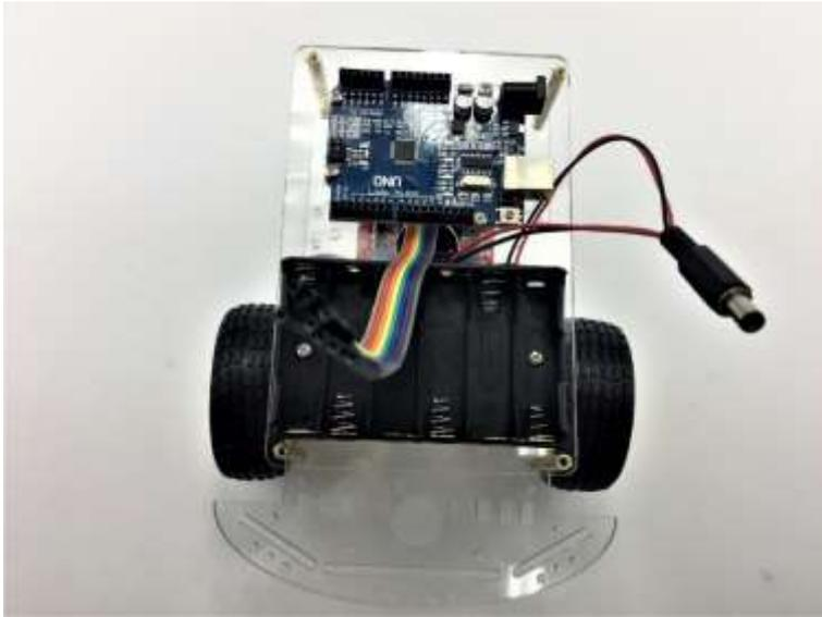
Mount the top acrylic chassis to the bottom chassis
