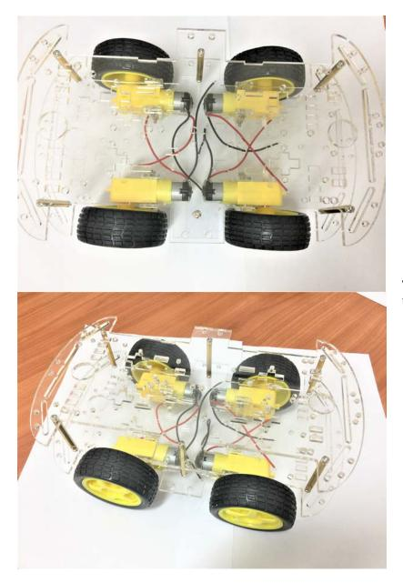
The last step is mounting the wheels on!
