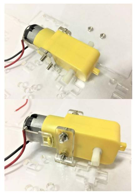
Then use two nuts to secure the screws
