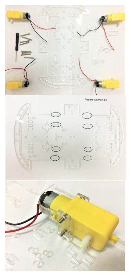
For each motor, we use two long screws to secure the motor on the chassis
