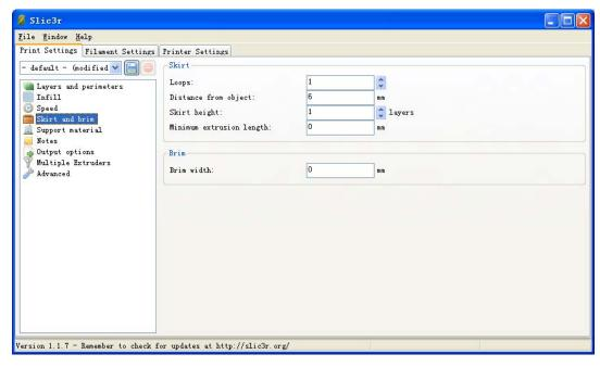
This setup is for the nozzle action in the beginning. It will a circle of lines around the product. We suggest you keep this setup because in the beginning, the nozzle will be in short of filament. After one circle. The filament feeding will be normal.
