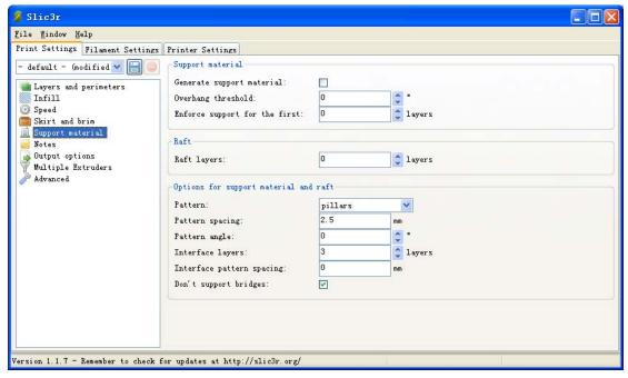
During the printing, there may be hollow parts or connection using bridge. If the bridge is too long, support is needed. Support is extra part, you can remove after the the printing is complete. Raft is the base layer during the printing. When printing on glass heat bed, raft is not recommended.
