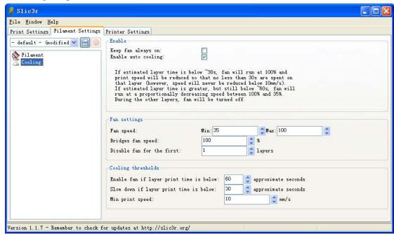
For cooling option, it's mainly used in printing small objects or printing hole parts. Otherwise, warpage will happenin printing big objects.
