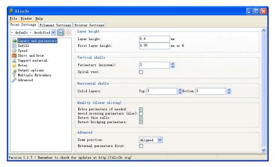
A. In layer setting, there are layer height and first layer height. Layer height means height for each layer during the printing. It's generally base on nozzle diameter. The higher the value, the coarser the product. The lower the value, the finer.
