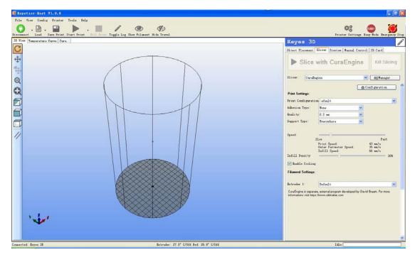
2)after setting up the language, we can set up configuration linking the printer and the software.
