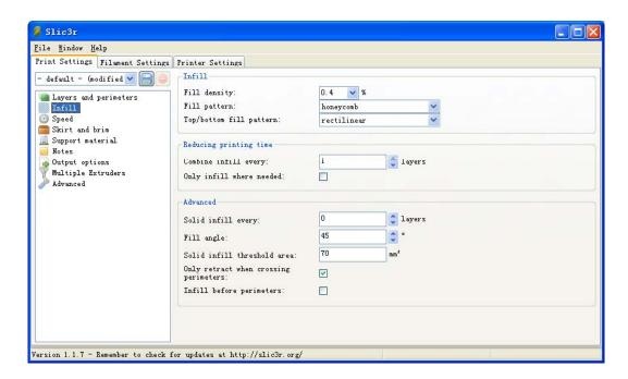
A. In the infill settings. One option is fill density, which means density of filament. For fill pattern and top/bottom fill pattern, you can choose freely as they don't affect product much.
