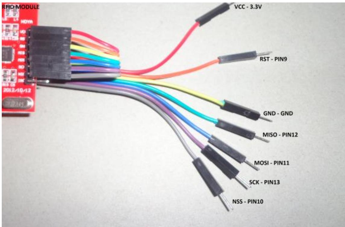
Once you have done that, upload the following code to the Arduino, and open the serial monitor. As instructed in the serial output, introduce your tag or card to the reader and you will see the data stored on it in a table.
