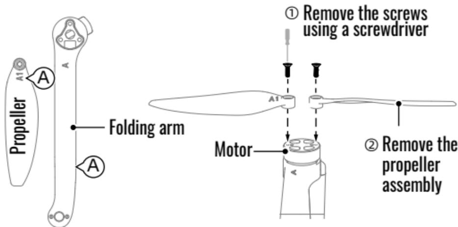
Remove propeller components in serial order. Operation in the opposite direction during installation. The propeller is divided into AB, corresponding to the letter on the folding arm. Please make sure it is installed correctly, otherwise it cannot fly.
