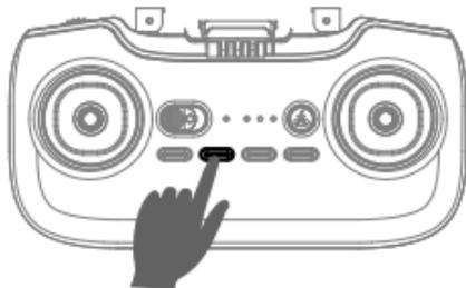
**Note:** Switch to high speed switch, obstacle avoidance function will be disabled.
