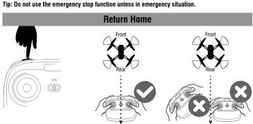
Press the "Return Home" button, the transmitter will sound "di", and the drone will fly back to the users. Pull down the Left Stick slowly to land the drone when the drone fly back and close to the user.
