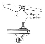
Remove: Turn out the screw, hold the propeller and pull out the propeller upward in the direction of the vertical motor.
