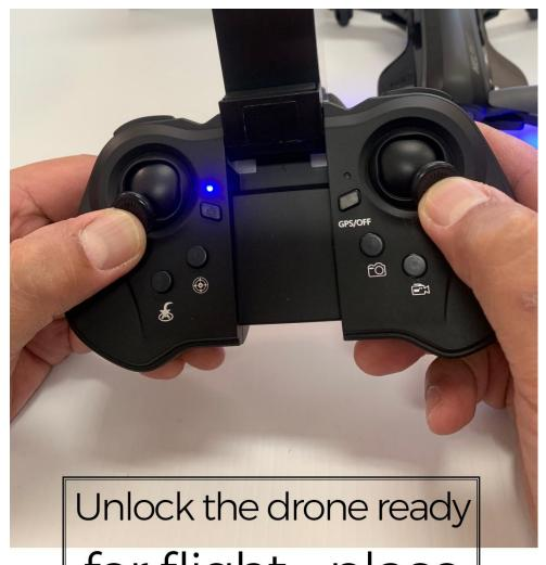
for flight - place & hold left hand joystick to bottom peft hand corner & right hand joystick to bottom right hand corner simultaneously
