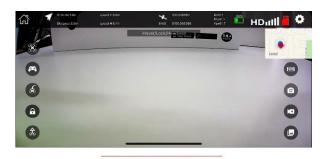
APP DEFAULT SETTINGS IS SET TO ONLY FLY ON STRONG GPS SIGNAL (MIN 9 SATELLITES). ENSURE TO USE OUTDOORS TO ACHIEVE THIS. To take off without waiting for strong GPS signal go to settings and change Take off on Good GPS signal to NO
