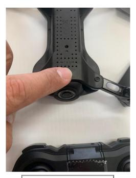
Power the drone on by pressing switch for 3 seconds
