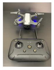
Now turn on the Remote controller by pressing the on/off button for 2 seconds.
