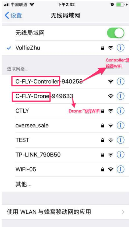
4. Please take note of the 6 digits unique number of the remote controllers Wi-Fi signal (as below picture, it is 940258), you will need these numbers when pairing the Remote controller with the drone.
