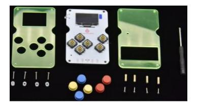
(2) Fix the GAMEPI game board and acrylic top board together with 4 M2\*10MM round-head screws, 4 white insulating column, and 4 M2.0\*11MM dual-pass copper pillars.
