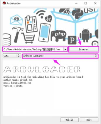
C. Press reset button on game machine, the COM port will change briefly, click the area arrow points to and set COM port. You'll find that com1 changes into com4, as shown below!
