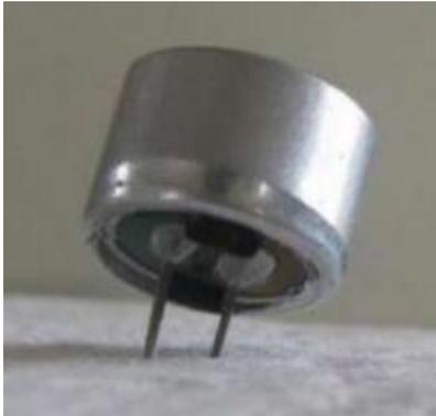
These microphones are widely used in electronic circuits to detect minor sounds or air vibrations which in turn are converted to electrical signals for further use. The two legs as shown in the image above are used to make electrical connection with the circuit.
