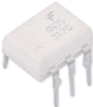
The 4N35 is a general-purpose optocoupler that contains a gallium arsenide infrared light-emitting diode, which is used to drive silicon phototransistors.
