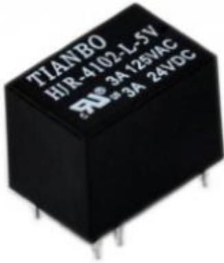
A relay is basically an electrically controlled mechanical switch with isolation function. Relays are used where it is necessary to control a circuit by a low power signal (with complete electrical isolation between control and controlled circuits), or where several circuits must be controlled by one signal. It's widely used in remote control, remote sensing, communication, automatic control, and electronic devices. It is one of the most important control elements.
