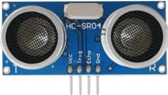
Ultrasonic sensor module HC-SR04 provides 2cm-400cm non-contact measurement function, the ranging accuracy can reach to 3mm. The modules includes ultrasonic transmitters, receiver and control circuit. Distance sensors work by sending pulses of light or sound out from a transmitter, then timing how long it takes for the signals to bounce off an object and return to a receiver (just like sonar).
