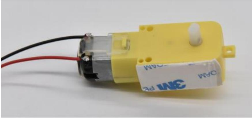
2. Press the motor to the baseplate, connecting the Dual Lock surfaces. Try to get the motors as straight as possible so your robot will drive straight.
