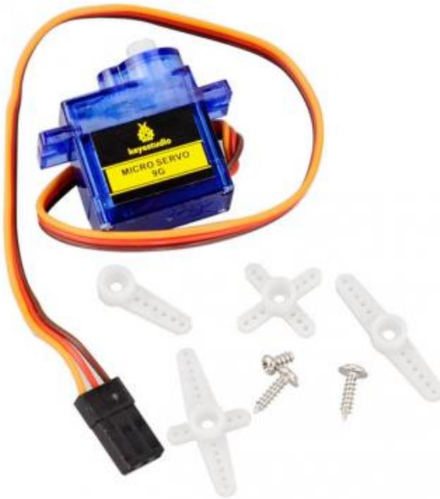
Included with your servo motor you will find a variety of white motor mounts that connect to the shaft of your servo.
