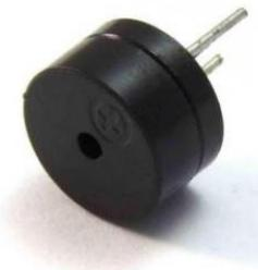
**POLARITY:** The buzzer is polarized. To see which leg is positive and which is negative, flip the buzzer over and look at the markings underneath. Keep track of which pin is where, as they will be hard to see once inserted into the breadboard. There is also text on the positive side of the buzzer, along with a tiny (+) symbol.
