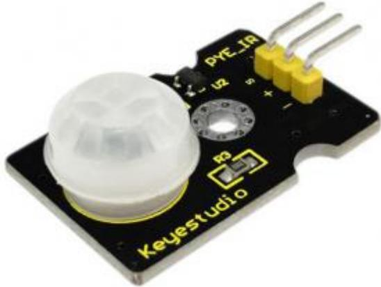
The Pyroelectric infrared motion sensor can detect infrared signals from a moving person or moving animal, and output switching signals. It can be applied to a variety of occasions to detect the movement of human body.
