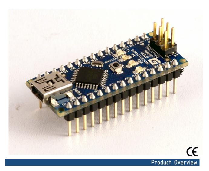
The Arduino Nano is a small, complete, and breadboard-friendly board based on the ATmega328 (Arduino Nano 3.0) or ATmega168 (Arduino Nano 2.x). It has more or less the same functionality of the Arduino Duemilanove, but in a different package. It lacks only a DC power jack, and works with a Mini-B USB cable instead of a standard one. The Nano was designed and is being produced by Gravitech.
