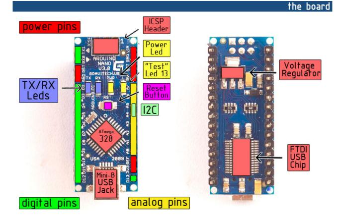
The Arduino Nano can be powered via the Mini-B USB connection, 6-20V unregulated external power supply (pin 30), or 5V regulated external power supply (pin 27). The power source is automatically selected to the highest voltage source.
