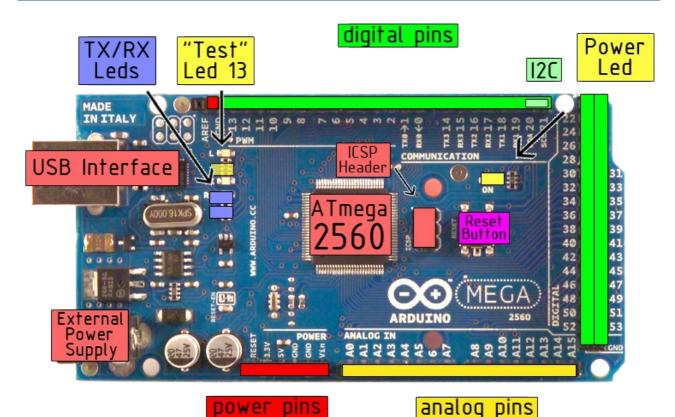
The Arduino Mega2560 can be powered via the USB connection or with an external power supply. The power source is selected automatically. External (non-USB) power can come either from an AC-to-DC adapter (wall-wart) or battery. The adapter can be connected by plugging a 2.1mm center-positive plug into the board's power jack. Leads from a battery can be inserted in the Gnd and Vin pin headers of the POWER connector.
