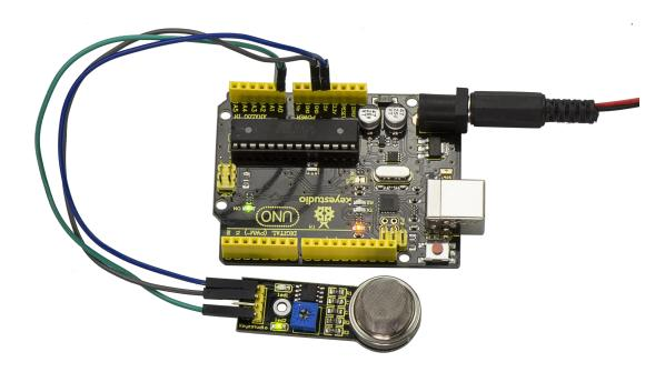
Done wiring and powered up, upload well the code, then open the serial monitor and set the baud rate as 9600, you will see the analog value.
