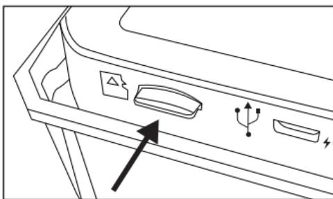
Insert the memory card as shown in the adjacent illustration. Push the memory card into compartment until it clicks into place.
