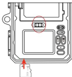
Insert U1 CLASS10 or above TF memory card in the memory card slot before switching on the camera and select, SETUP mode to adjust settings.
