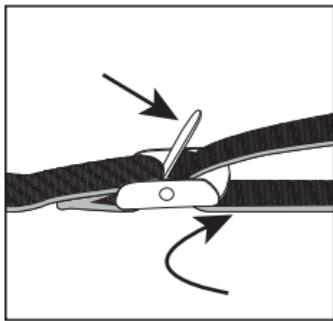
Position the Wildlife Camera as desired and pull the loose end of the securing strap tight until the camera is firmly secured.
