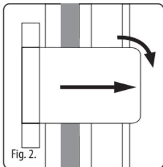
A fixing for a padlock is provided between the two locking brackets, allowing the camera to be securely locked.
