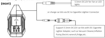
Note: The 12V DC output voltage is range between 9V~12.6V, maximum output current is 15A. DC output voltage drops while battery capacity drops due to chemical characteristics of the battery. If your appliance is not built-in input voltage stabilizing function, it may shutdown when input voltage is too low, please unplug your device from the unit in time And please charge the unit in time.
