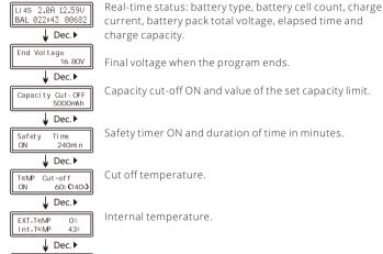
Temperature probe needs to be connected to show external temperature.
