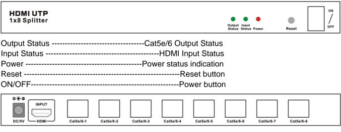
DC/5V ------DC 5V Input Port HDMI Input ------HDMI Input Port Cat5e/6-1------Cat5e/6-8: RJ45 Output Ports
