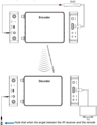
control is  $\pm$  45°, the transmission distance is 0-5 meters; when the angle between the IR receiver and the remote control is  $\pm$  90°, the transmission distance is 0-8 meters.
