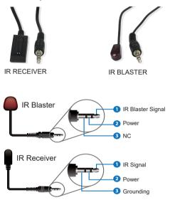
Connection diagram of using IR cables.
