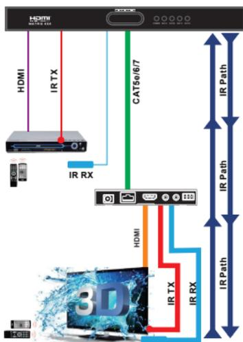
The matrix is not only a switcher and extender of multiple HDMI signals to multiple HDMI receivers located remotely, it also passes IR control signals through the IR call-back system to the matrix and HDMI sources for full, independent control of all connected inputs from output locations.
